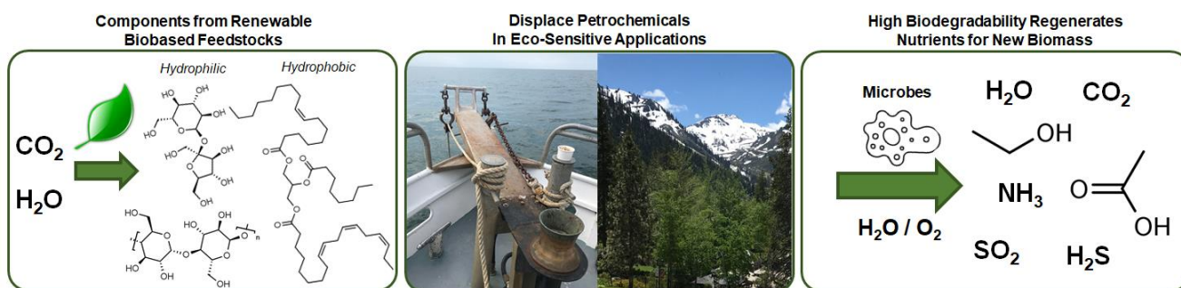
Figure 1: Lifecycle of environmentally acceptable lubricants (EAL) from renewable beginning to biodegradable ending
